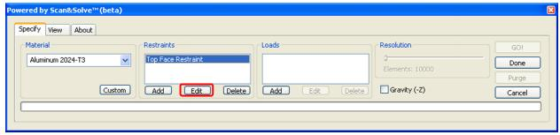
[**Edit**] displays the Restraint Editor, allowing the selected restraint to be modified:
