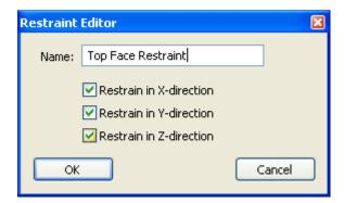
[Restrain in X-direction] the face will be fixed in the X-direction, but may be free to move in the other directions unless they too are restrained.
